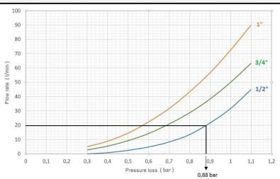
The graphic is prepared according to the conditions specified in EN 1567 standard. (Input pressure 8 bar - Output pressure 3 bar)
