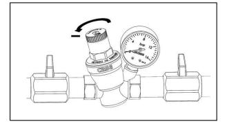
After closing the inlet and outlet valves, remove the spring pressure by turning the adjustment key in the minus (-) direction.
