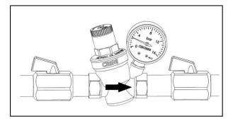
Care should be taken to ensure that the arrow mark on the product's body is in the direction of the water flow while the product is connected to the installation.
