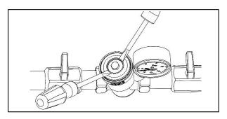
Remove the cartridge by lifting it from under the metal disc with the help of two screwdrivers or with a similar device.
