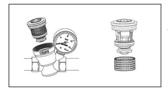
If the filter needs to be cleaned, remove the filter, clean it and put it back on the cartridge. Then insert the cartridge into the product. If the cartridge needs to be replaced, replace the old cartridge with the new cartridge you supplied.
