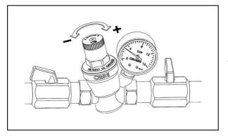
If necessary, adjust the pressure value to the desired value by turning the adjustment key clockwise (+) to increase pressure and counterclockwise (-) to decrease the pressure.
