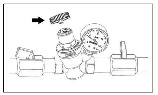
Re-insert the pieces you have previously removed and tighten the cover with the wrench. Observe the manometer and adjust it with the adjusting key to the desired pressure value.
