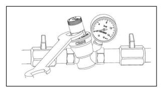
With the help of a tool such as a wrench, remove the cover by turning it clockwise.
