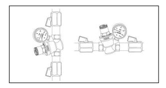
The installation of the product can be made vertical or horizontal.
